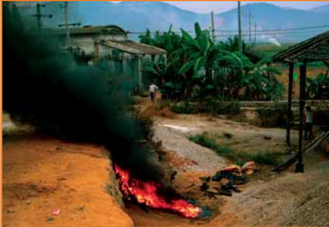
Open burning of wires and other parts are common to recover metals such as steel and copper. Dioxins and furans can be expected due to the use of PVC and brominated flame retardants. (photo: BAN)
